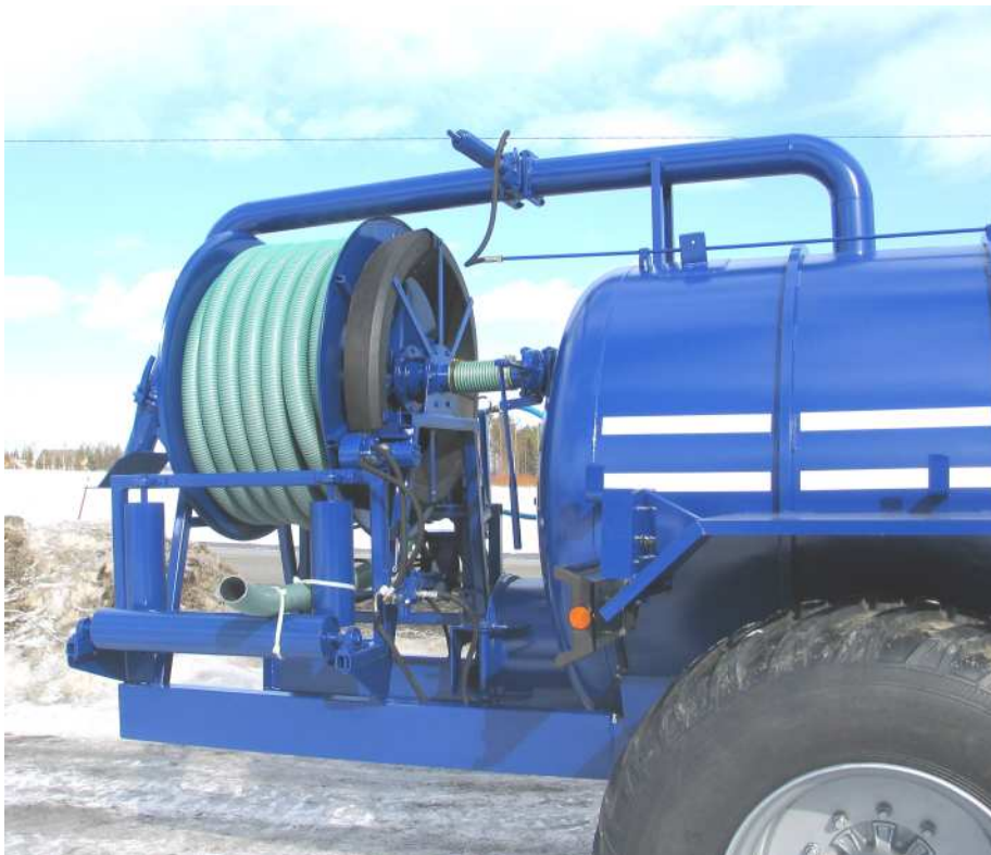
Hose reel for suction hose. The reel is made for Ø 76 mm hose, maximum length 30 m.
